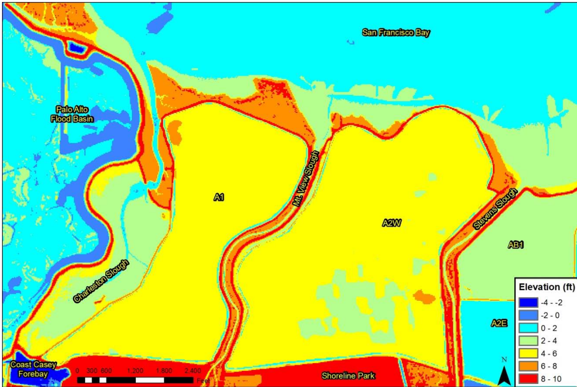
Figure 3-5. Topographic and bathymetric map showing the future ground surface elevations used to represent the Mountain View Ponds and surrounding ground in the model
